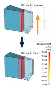
New cylindrical (top right) and ring-shaped shrink fit windows have been introduced. They support
